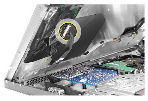
Replacement Note: If replacing the display panel, disconnect the LVDS cable from the panel before returning the module to Apple. Transfer the LVDS cable and the inverter cable (previous step) to the replacement panel. A replacement panel includes the display panel mounting brackets, the mylar tape, the foam strips and gaskets, the display temp sensor, and the display temp sensor cable.
